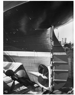
RMS Olympic 's rudder with central and port wing propellers; [4] for scale note the man at the bottom of the photo. [37]
