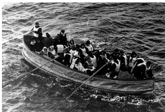
A collapsible lifeboat with canvas sides
