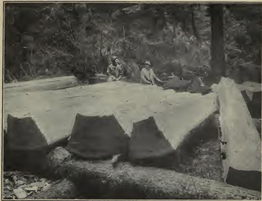
"Rived" Spruce Logs. Note the Straight Grain. The Logs Shown are
