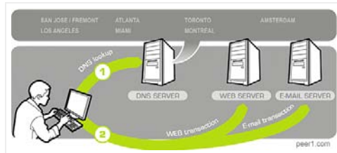
FIG.2 —If the DNS lookup finds a missing or corrupted entry for your website, the user is prevented from navigating to your website. The DNS lookup directory is a single point of ultimate power and control over the operation of the Internet. It cannot be permitted to be put into private hands where censorship of one's adversaries is an inescapable temptation. Power corrupts. Absolute power corrupts absolutely.
